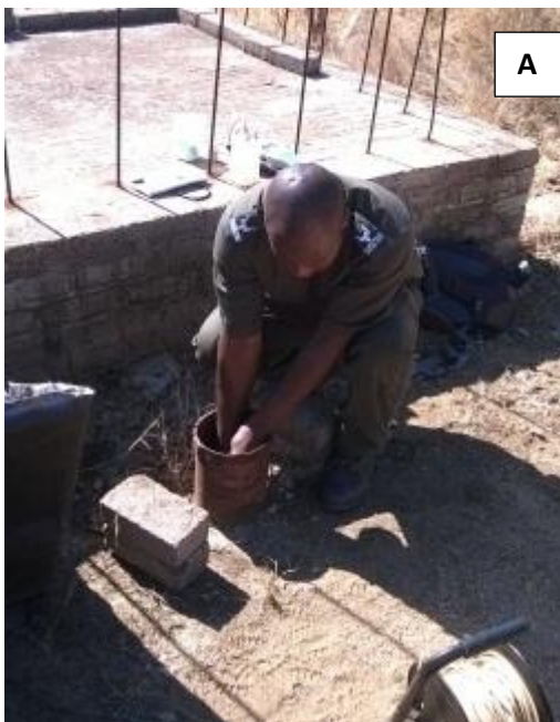
Figure 6.5 Using a baler to obtain a water sample for hydrochemistry during a hydrocensus (A) while (B) depicts a dyke intercepting the river bed along the Groot Letaba.
