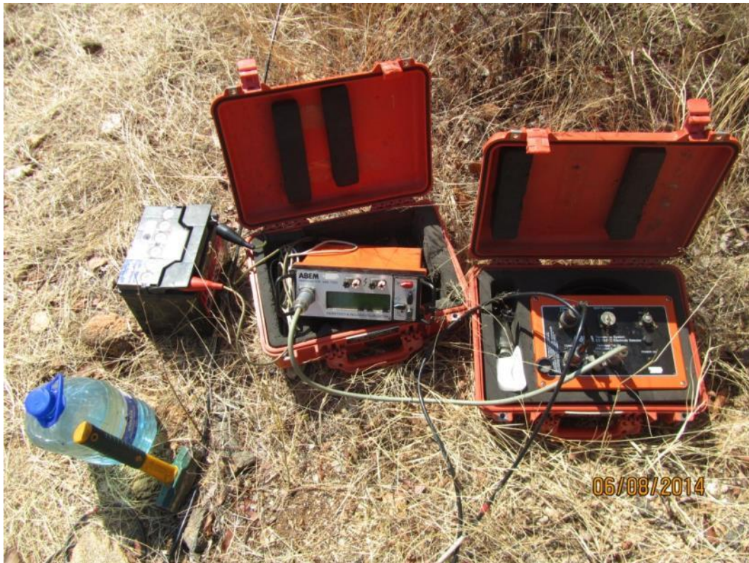
Figure 6.1 The ABEM Terrameter used to measure resistivity of subsurface geology.
