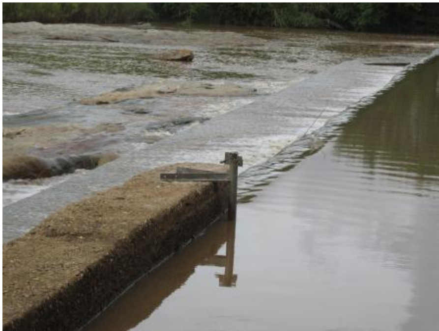
Figure A2.II: Solinst Level Logger Installation at the Mahale weir to record streamflow head, installed on 22 April 2015.
