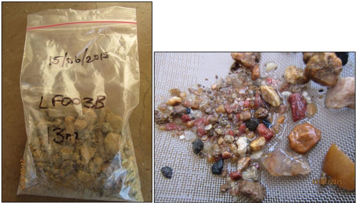
Figure A3.II: Example of a borehole log collected before analysis and how samples look after rinsing.
