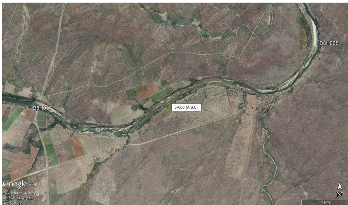
Figure 6-1 Location of the Mahale Weir (B8H007) and Letaba Ranch Weirs (B8H008) which are used in the mass balance approach to determine Transmission Losses at the study site.
