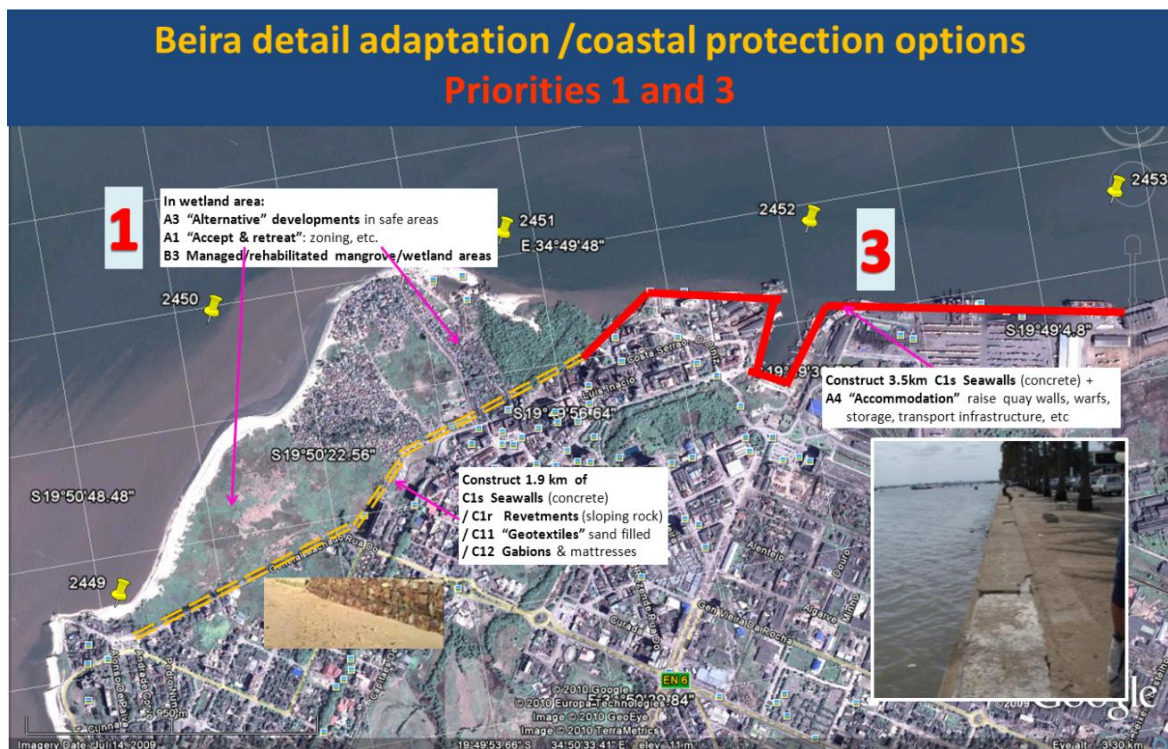
Figure 8.2: Western Beira. Adaptation / coastal protection options based on general criteria, local site characteristics, current use / "value"
