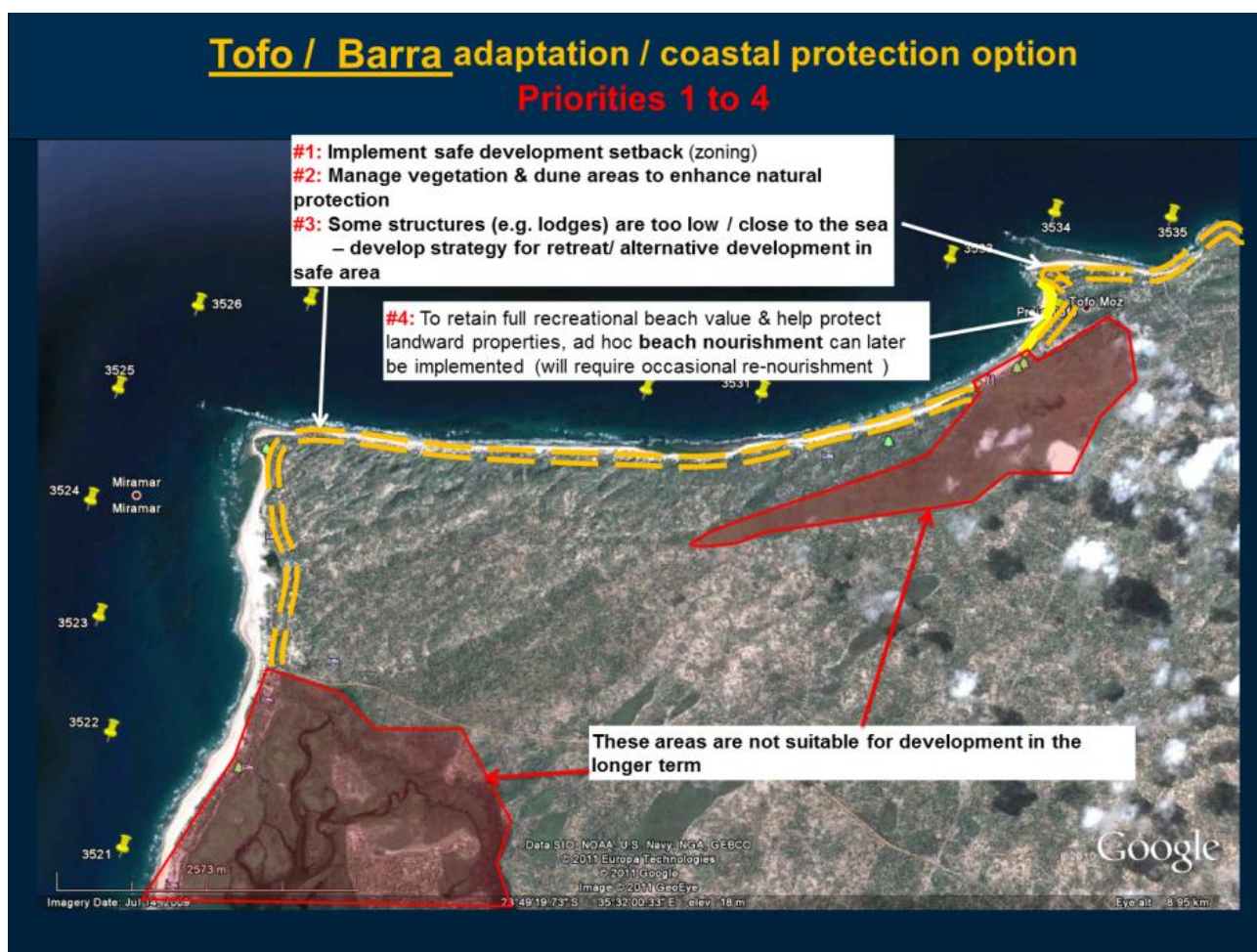
Figure 8.12: Tofo & Barra. Recommended adaptation /coastal protection options
