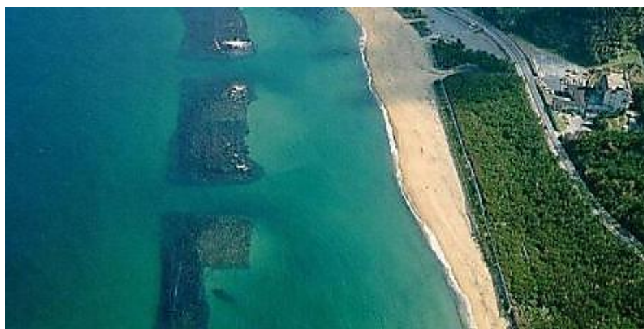
Figure 7.10: Example of beach accretion through submerged artificial reefs
