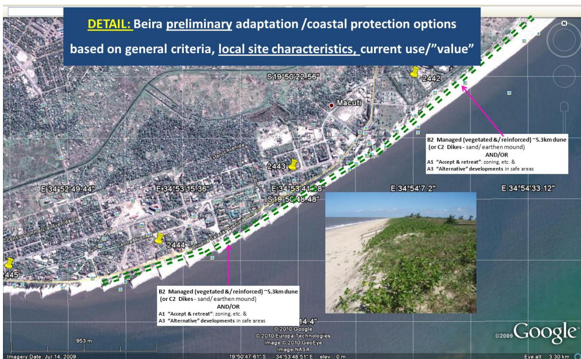
Figure 8.5: South-eastern Beira. Adaptation / coastal protection options based on general criteria, local site characteristics, current use/“value”.
